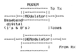
Fig 1: The Modem converts digital information into audio for the TX and audio into digital fot the RX.
